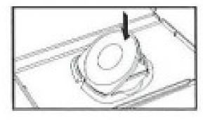
Place the disc as shown, gently pressing downwards until it clicks into place. Storing the disc incorrectly may result in damage.
