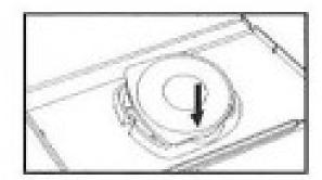
Push down one side of the disc as shown and gently pull upwards to remove it. Using excess force to remove the disc may result in damage.
